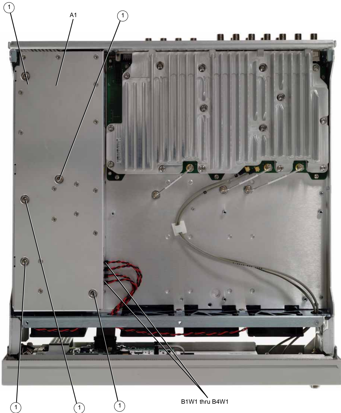
Figure 3-14 A1 Power Supply
